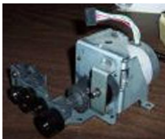
Fig. 2. Stepper motor with gear assembly
