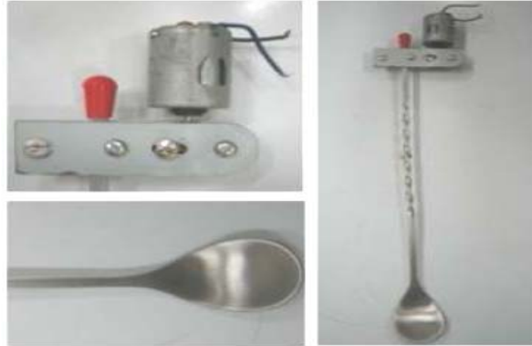
Figure 5: The Mixer comprising the DC Motor and the Bar Spoon
