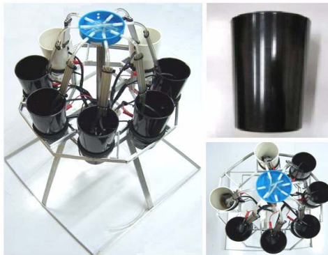
Figure 4: Prototype's dispensers for the seven ingredients.
