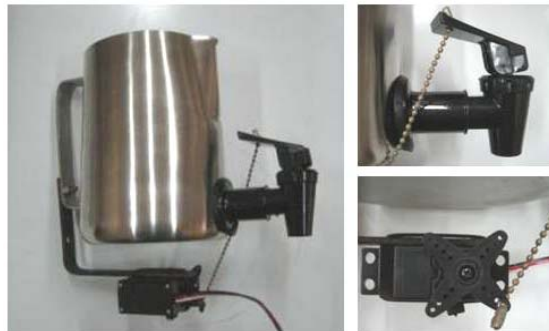
Figure 6: The Mixing Container comprising of the valve and the servo motor
